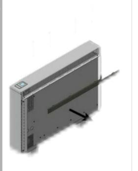
Step 6: Unscrew the anchoring bracket at the rear and remove it.
