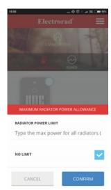
The Smartbox will communicate with the radiators to ensure the set limit isn't exceeded. Within the configuration option you can also set the level of priority for each radiator (dictating which radiators will receive the heat quickest within the house and which are less important) and you can also name the radiators if required.
