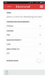
The Smartbox will first turn off the lower priority radiators unless there is a considerable difference between the set point temperature and the ambient temperature, this is to ensure the temperatures requested are maintained in your home at all times.
