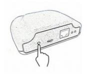
The Smartbox unit communicates with the radiators via radio frequency, and with the router via an Ethernet cable (supplied).
