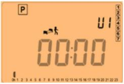
Now, adjust the hour of the first step of the program with  $(\blacktriangleleft-)$  or  $(\triangleright+)$ ,
